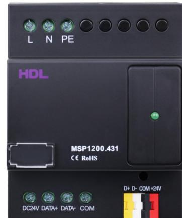
HDL-MSP1200.431 is a power supply module. The module can supply DC24V voltage , 1200mA current. It has 2 kinds of connection types, the total current is 1200mA
